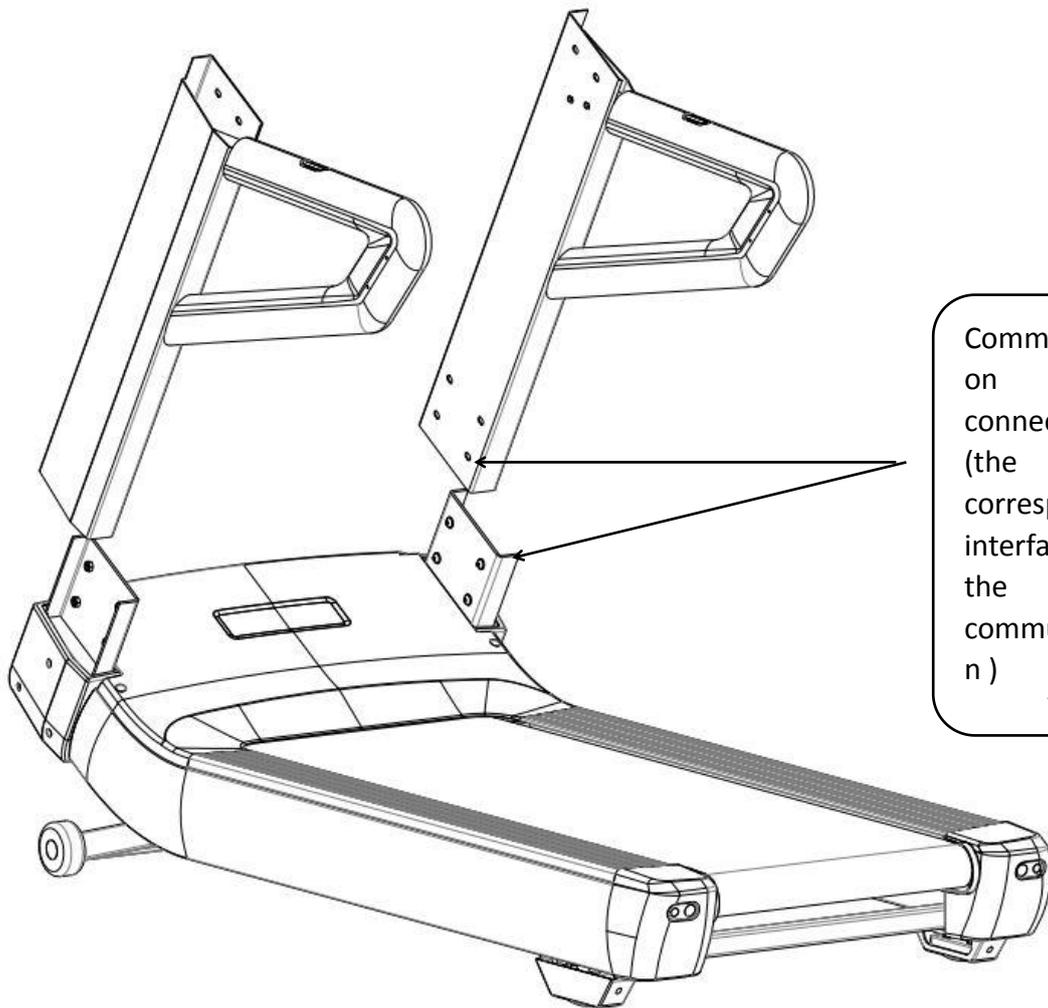
Communication line connection (the only corresponding interface of the communication)
