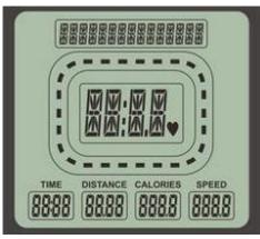
The main interface is used to display device name, time, distance, calories, speed,
